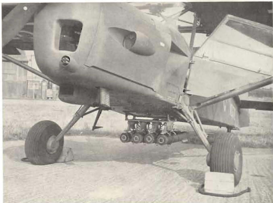
A light series bomb carrier can be fitted to the Mk. 9 to take advantage of tactical opportunities, or to train aircrew in light bombing. In this case four 4" flares are carried for target marking.
