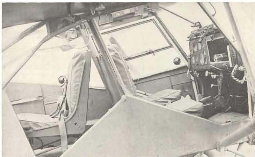
The two doors on the starboard side of the Mk. 9 afford easy entry to both front and rear of the cabin. The starboard half of the instrument panel houses an M.F. radio (not fitted in photograph). Door jettison handles are striped for identification.
